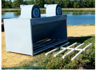
The LAGOON MASTER out of the water, ready for installation. Weighing less than 1100 pounds (499 kg), it is simple to install because it floats in less than 5 feet (1.5m) of water depth. It can be tethered to the bank or out in the lagoon, whichever is preferred.
