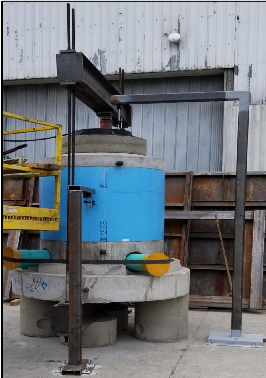
Pic.3: Bridge assembly and standalone arms for Gauges
