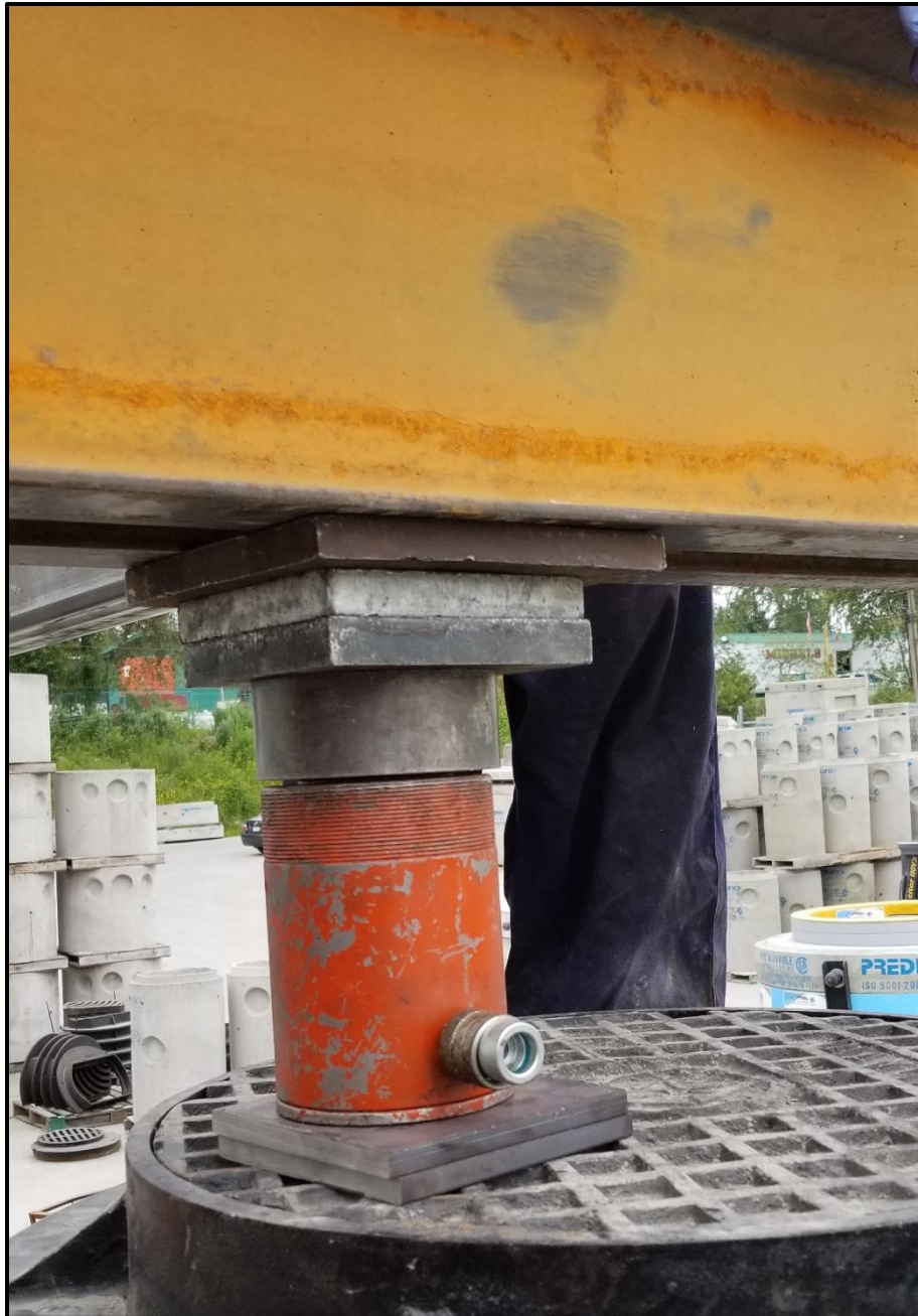
Pic.5: Hydraulic ram set up
