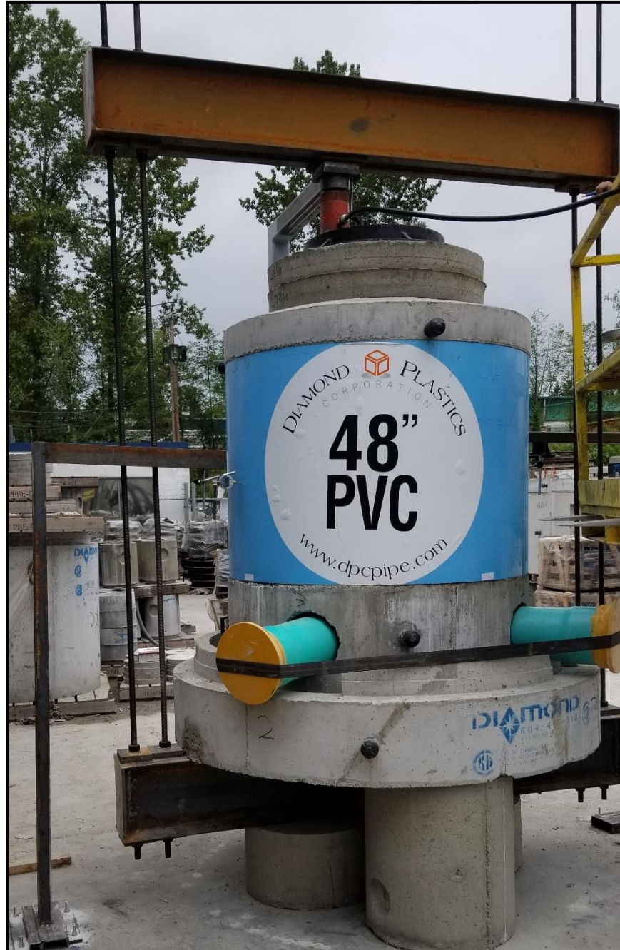
Pic.1: Manhole Test Assembly
