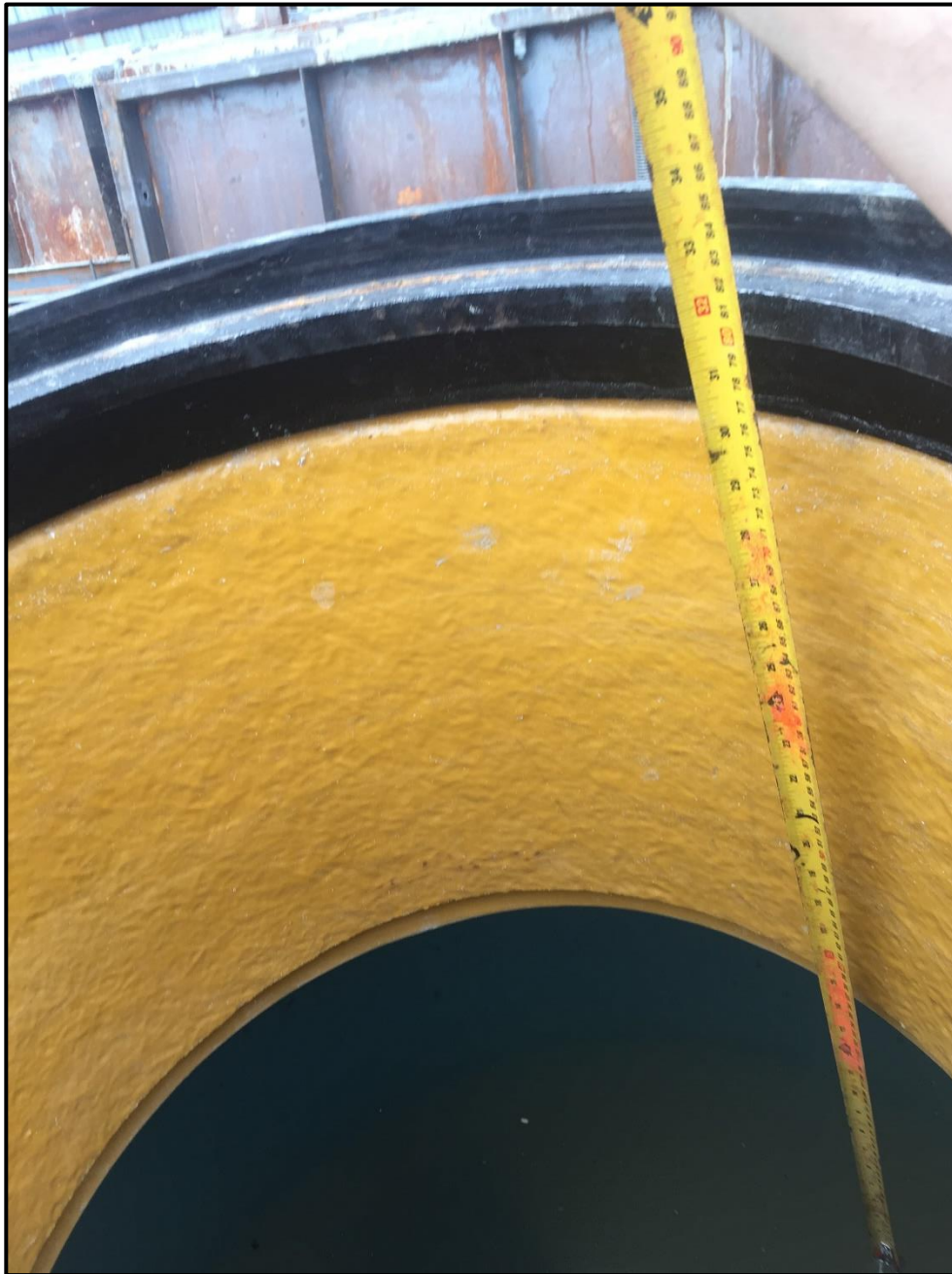
Pic.4: Filled water up to a depth of ~1000 mm.
